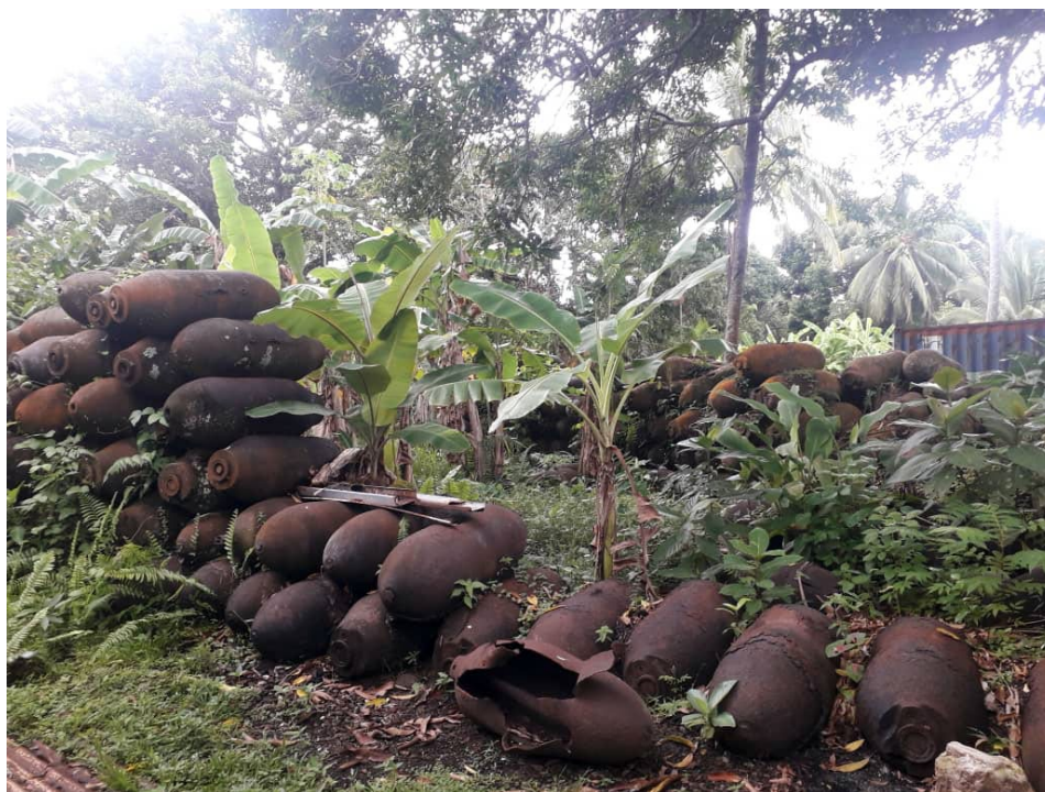
Figure 11: Near Oro Bay, Papua New Guinea, March 2023. Note the bomb in the center foreground, which appears to have ruptured from internal pressure, perhaps as a result of CK polymerizing. Photographed by Basil Tindeba Emimie
